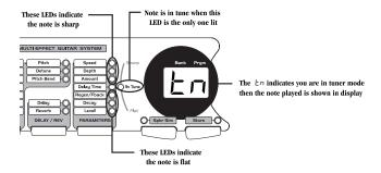
he tuning reference on the GS30 has been set to A=440 (concert pitch) from the factory. You may change the uning reference for drop tunings by rotating the Data Wheel at any time while in the tuner mode. Your tuning hoices are  $\overline{A}$  (standard tuning),  $\overline{A}$  (1/2 step flat),  $\overline{A}$  (whole step flat), and  $\overline{A}$  (one and 1/2 steps flat). ressing any footswitch will exit the tuner mode and return you to the performance mode.
